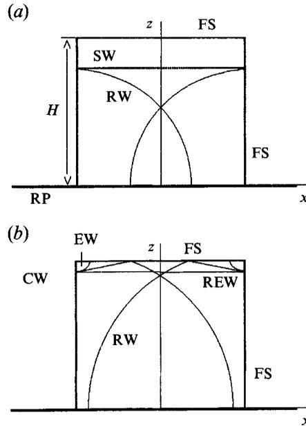
FIGURE 7. Impact by a finite liquid cylinder (a plane case is shown). (a) The wave pattern at the initial stage when the presence of the upper free surface does not affect the flow: FS, free surface; SW, shock wave; RW, relief wave; RP, rigid plate;  $H$ , length of the cylinder. (b) Reflection of the shock wave at the upper free surface of the cylinder: REW, reflected expansion wave; EW, edge wave; CW, compression wave.
