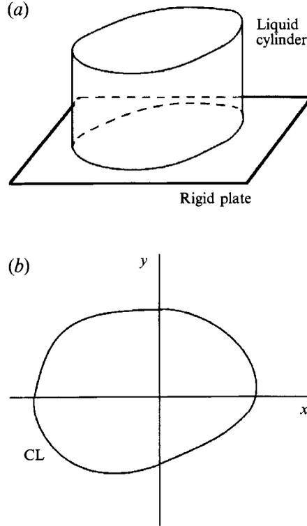
FIGURE 6. Impact of a plate on a liquid cylinder of arbitrary cross-section. (a) General view at the initial moment. (b) The bottom view: CL, contact line between the liquid free surface and the plate.
