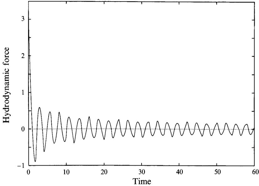
FIGURE 5. Hydrodynamic force  $F(t)$  on a plate impacted by an axisymmetrical jet.
