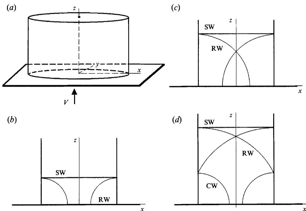
FIGURE 1. Impact of a plate on an half-infinite liquid cylinder. (a) Initially, liquid is at rest and occupies a cylinder  $z > 0$  of arbitrary cross-section. The side boundary of the cylinder is free. (b–d) The wave pattern at the initial stage of the impact (plane case): (b) SW, shock wave; RW, relief wave produced at the impact moment. (c) Interaction of the relief waves. (d) CW, compression wave produced by the relief wave reflection in the free surface.
