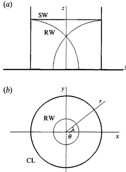
FIGURE 4. Impact of a plate on a liquid circular cylinder. (a) The side view of the wave pattern at the initial stage of the impact (axisymmetric case): SW, shock wave; RW, relief wave;  $r$ , radial coordinate. (b) The bottom view: CL, contact line between the liquid free surface and the plate; relief wave, RW, converges to the centre point.
