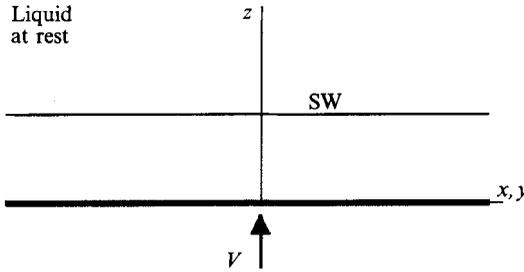
FIGURE 2. Creation of an acoustic shock, SW, by impact on a liquid half-space.
